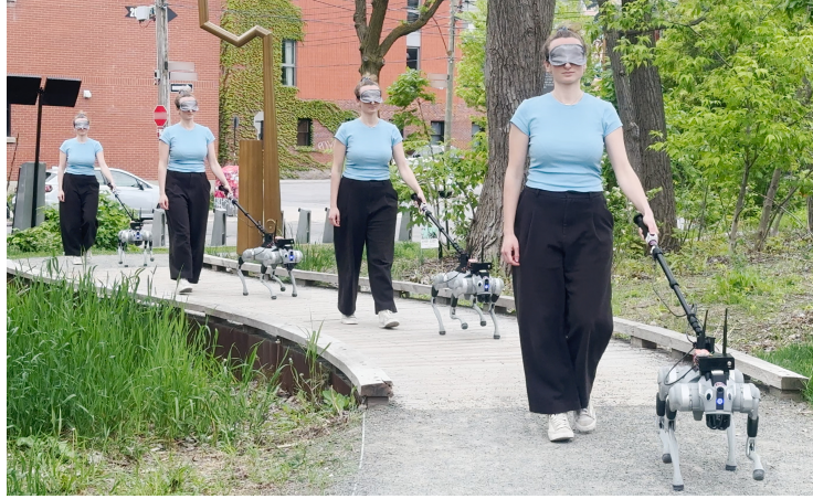
Figure 1: Milo autonomously guides a handler along indoor and outdoor paths while avoiding obstacles and oncoming pedestrians, adapting to the handler’s position, desired walking speed, and turn commands. The project is released as open source.
